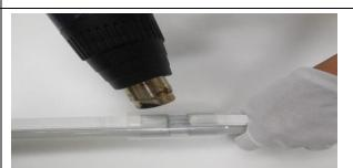
8. Usng the heat gun,gently heat the heat shrink tube until it is sealed into place.Seal both ends of the heat shrink tube with silicone sealant glue.This will ensure that the end cap is securely attached and the connection is impermeable to moisture.
