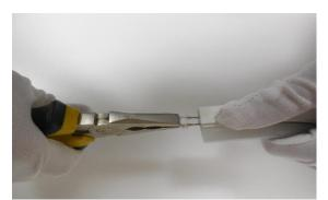
4.Using a pliers hold connecting pin and insert he pointed end of the electrical pin into the endof neon flex.The pin must be installed on the right side or it will not line up with the end cap on the power cord.
