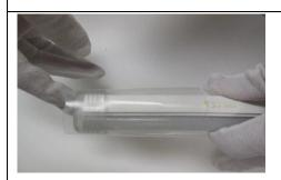
3.Locate the heat shrink tube and slide it onto the LED neon flex.Allow the heat shrink tube to extend past the free end of the end cap approximately 1/4 to 3/8 inch
