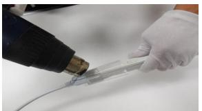
8. Using the heat gun,gently warm the heat shrink tube until it shrinks into its final resting place,after completed,seal around both ends of the shrink tube with silicone sealant glue.
