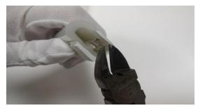
3.Trim loose wires.Don't forget to trim any loose wires hanging out,flush to the PVC with sharpe side cutters or scissors.
