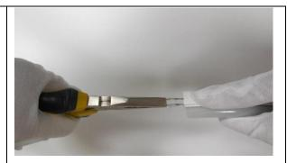
2.Position the connecting pin so as to insert into one selection of LED neon flex with pick/awl tool.Gently push the pin into the wires
