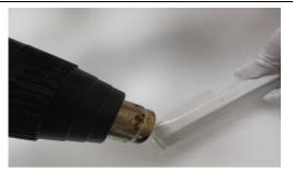
4.Usng the heat gun,gently heat the heat shrink tube until it is sealed into place.Seal both ends of the heat shrink tube with silicone sealant glue.This will ensure that the end cap is securely attached and the connection is impermeable to moisture.
