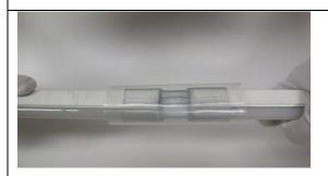
7.Location the heat shrink tube to the joint, Allow the heat shrink tube to extend past the free two ends of the straight connector approximately 1/4 to 3/8 inch
