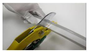
2.Cut at cutting mark using heavy scissors(Recommended using garden pruning shears,hose cutters or box cutter).Be sure to cut the line square and not on an angle
