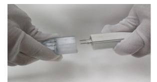
6. Aligning the pins with the receptacle holes in the power cord cap,gently push the power cord into place
