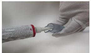
5.Using silicone sealant glue, seal the power cord cap
