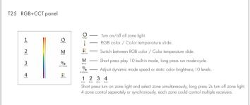
Note: After touch power key to turn off light, long press power key for 5 seconds will turn on or turn off tone.
