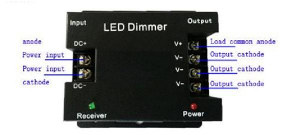
DC+: Power supply + (voltage12v-24v)
